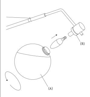
4. Insert the light bulb then gently mount the diffuser screwing it back to the metal ring.
