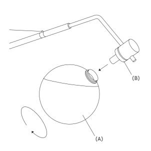
3. Unscrew the diffuser (A) while holding the metal ring (B).
