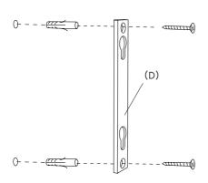
Mount the wall mounting (D) to the wall with two appropriate screws and plugs. Always use correct screws and plugs for the mounting surface.
