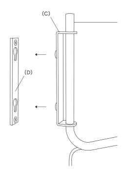
2. Attach the lamp body (C) to the wall mounting. Make sure that both fixings on the lamp body are inserted in the slots on the wall mounting.
